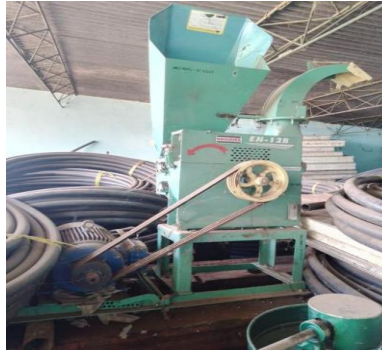
Silage Cutter Stored in an Office
