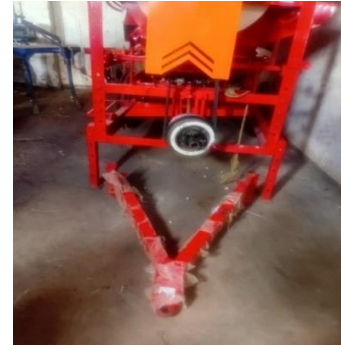
Multi Crop Thresher without Drawbar – Lusitu FTC Incompatible Drawbar
