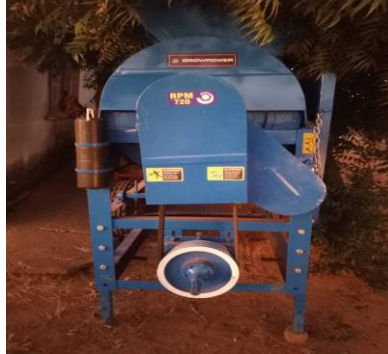
Multi Crop Thresher without Drawbar – Lusitu FTC Incompatible Drawbar
