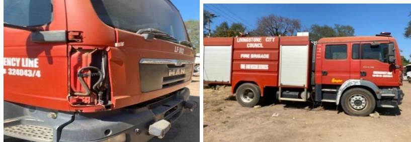
Fire truck with damaged and missing parts
