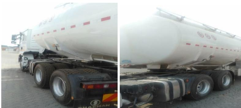
*Fuel tank trailer not protected by mudguards from the rear horse wheels*
